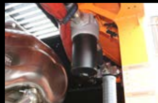
Drain filter for travel and mulcher circuit
